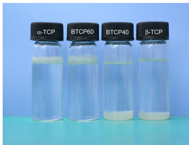
Fig. 5. The sedimentation test results of the monophasic and biphasic TCPs.
